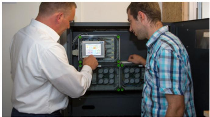
The XV102 HMI/PLC can be operated easily via the touch screen, a laptop is not needed for the configuration.
