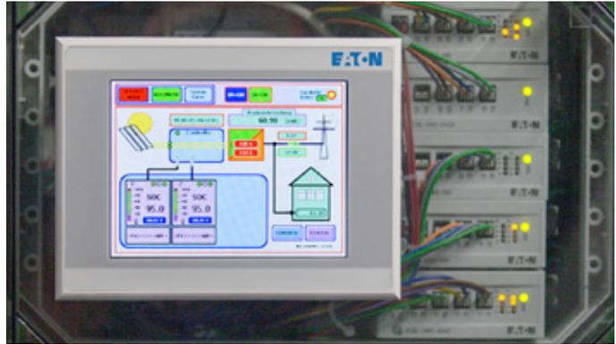
The Eaton HMI/PLC comes with several interfaces and the SmartWire-DT connection technology simplifies the wiring.
